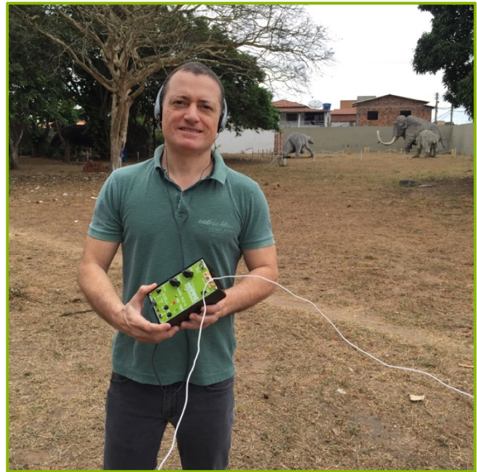
Figure 2: Here I am in 2015 conducting one of the first VLF-3 field tests. The two wires: one as ground connection (left) and antenna (right). This place is at Antares Observatory area (don't panic with some pre-historic animals in the background near the power lines).
