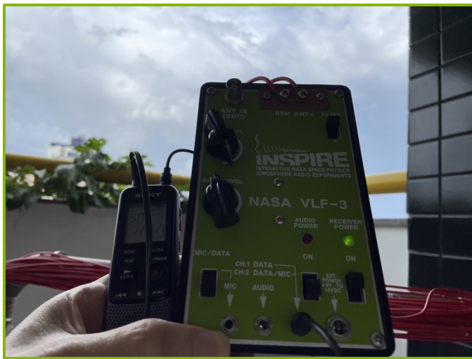
Figure 5: A cloudy sky in the background. The loop antenna with red wire, the digital recorder, with headphones and data cables on the left, and the VLF-3 turned on.
