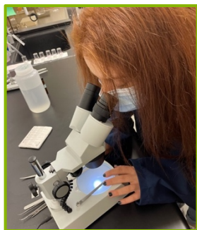
Figure 3: Electrode preparation – Michelle cutting carbon fiber microelectrode under the microscope
