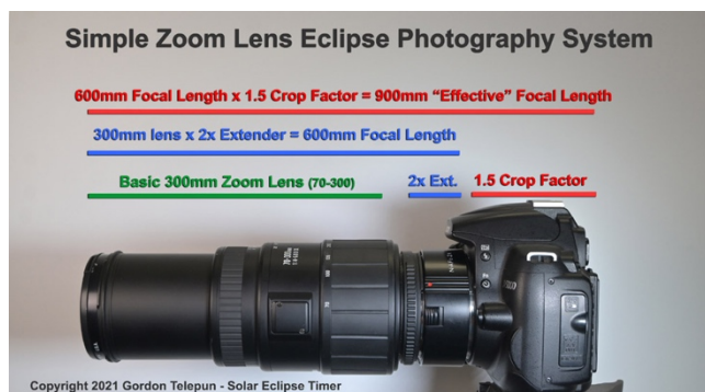
Figure 5. When this lens is zoomed all the way out, the 2x extender and the 1.5x crop factor make the system work at 900mm. This system would be best used at a focal length of 750mm. This would be achieved by taping down the zoom barrel at the 250mm setting.
