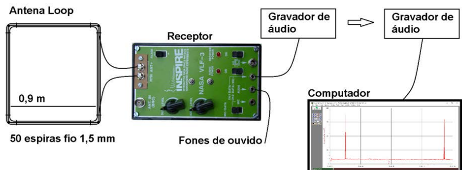
Figure 4: My VLF station main parts: loop antenna, receiver, headphones, audio recorder, and the laptop with Radio-SkyPipe and Spectrum Lab Software.
