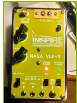
Figure 1: INSPIRE VLF-3 Receiver Front Panel
