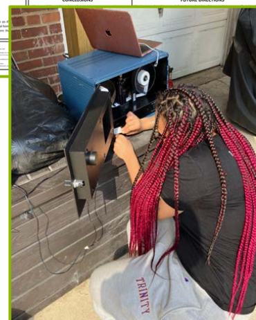
Martha calibrating the Aethalometer to ensure accurate BC monitoring.
