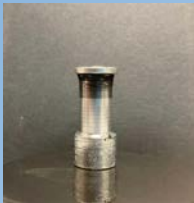
Fig. 1. Spun CNTY on the spool
