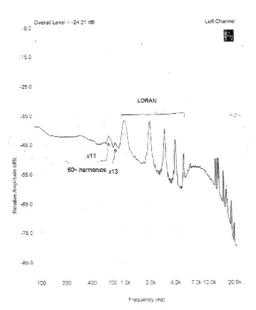
MISSION 337-A I used the 120-foot long wire antenna with a westward orientation. In this mission I used the RS-4 INSPIRE receiver. I detected a lot of very strong tweeks. The spectrum is shown in the following figure. Note the twin peaks at approximately 2 kHz. The first at 1.9 kHz is caused by the strong tweeks while the second at 2 kHz is a Loran component. The tweek energy is better represented in the Gram spectrograph, which follows. Note the strong component at about 1.9 kHz.
