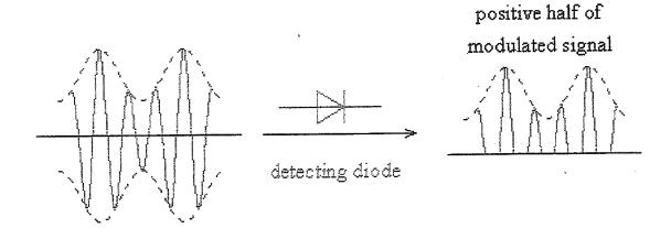
When the positive portion of the wave is averaged over time, it reproduces the original sound wave that the radio station used to modulate its carrier frequency wave. If it is strong enough, that wave can drive a speaker or recording device just as any incoming radio wave in the audio range would.
