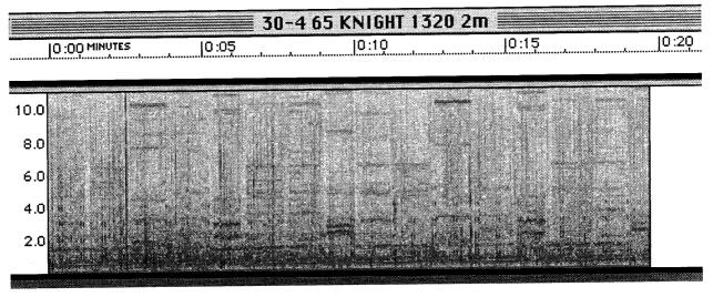
A 20 second sample starting at 1320 showing details of OMEGA. Three stations are visible: a strong dash at about 3 seconds, a weak dash at about 7 seconds and a slightly stronger dash at about 8-9 seconds. Dashes which appear at frequencies below 10.2 kHz are the result of aliasing.
