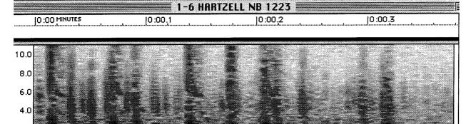
1224:03 UT Closeup of a burst of tweeks with hooks at just below 2 kHz and also prominent hooks at the second harmonic just below 6 kHz.
