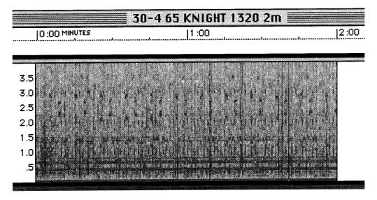
The above file using a 0-4 kHz frequency range. The ISTOCHNIK signal should appear as a series of dashes 10 seconds long indicating electron gun operation separated by 10 seconds of no signal. No signal is apparent at 1 kHz, 2 kHz or 3 kHz.
