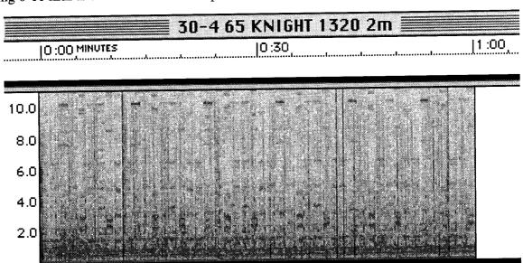
The first minute of the data file shown earlier. At this time scale, OMEGA is more recognizable. Note that the file name does not change even though the time interval has been cropped. You have to look at the time bar to see the length of the spectrograph in the image.
