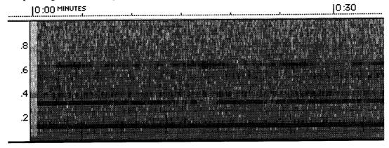
This spectrogram just shows the frequency range up to 1 kHz, which is where the noise seems to be found. Large fan motors would certainly put our a pretty strong electromagnetic signal with frequencies related to the rate of revolution of the fan motor.
