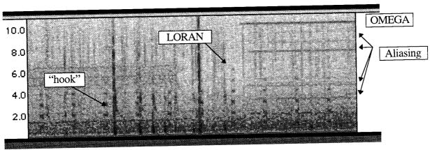
Finally an image starting at 1320:02 UT showing a strong tweek between .2 and .3 seconds. Tweeks can be identified by the "hook" at around 2 kHz. LORAN signals, a navigational aid, sound like a clacking noise and show up on the spectrograph as a vertical series of dots occurring periodically.
