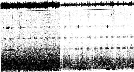
The above figure shows the effect of the recorder limiter. It was out in the first part of the recording up to about time 50 Sec then turned on. After the limiter was turned on, note the appearance of the faint signals at 1411, 3564 and 3693 HZ. The recorder was in saturation with limiter off and the above signals were not evident.
