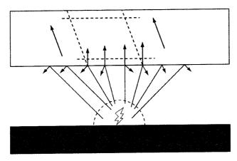
The lightning stroke causes a radio disturbance that travels outward in all directions. When the signal encounters the ionosphere, some is reflected and some is refracted. The refracted waves are formed into a beam (horizontal dashed line) which then follows the Earth's magnetic field (up to the left).
