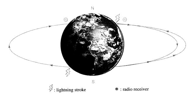
The curved lines represent Earth's magnetic field lines. The arrows indicate the direction of travel of the radio waves. The left show lightning originating in the Southern Hemisphere which is received in the Northern Hemisphere as a short whistler. On the right is lightning in the Northern Hemisphere which is heard, after the radio signal makes a round trip, as a long whistler.
