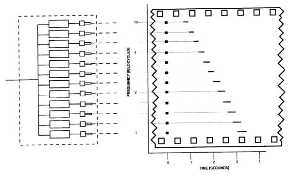
Sound spectrograph consists of a set of filters (rectangles) which each pass a narrow band of wavelengths. Each filter is connected to a small neon lamp (squares). A strip of photographic film is passed under the set of lamps. The click of nearby lightning appears on the film as a vertical row of spots (at 0 seconds). A whistler creates the diagonal row of marks as the higher frequencies arrive first followed in turn by the lower frequencies.
