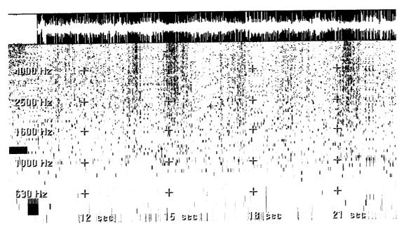
This image is the first few seconds of the operation in high resolution. Note the hum near 630 HZ and the high noise levels below 1 kHz.
