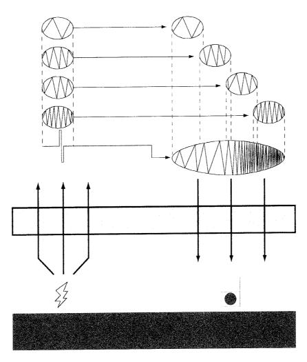
The radio signal from the lightning stroke at the left is heard immediately by the receiver at the right as a click (as illustrated by the rectangular waveform above the lightning stroke) composed of the variety of waveforms shown above. In the ionosphere (gray area) shorter wavelengths (higher frequencies) travel faster than longer (lower) which results in a whistler heard seconds later at the same receiver.
